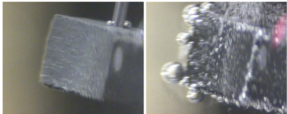
Fig. 6 Sintered Ta anode during cyclic voltammogram (sweep rate 100 mV s -1 ) at potentials <9 V during blocking (left) and with gas evolution (right)
